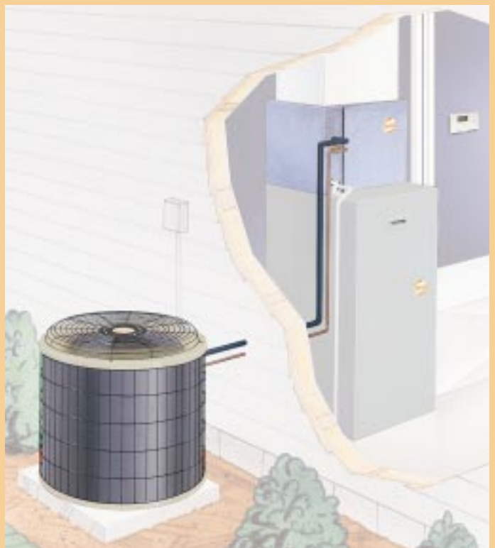
Central Air Conditioner and Evaporator Coil System
